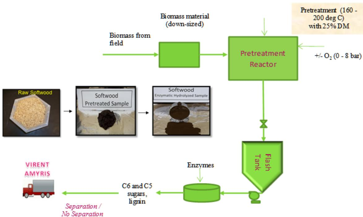
Figure 1: Schematic of the pretreated hydrolysate supply chain
