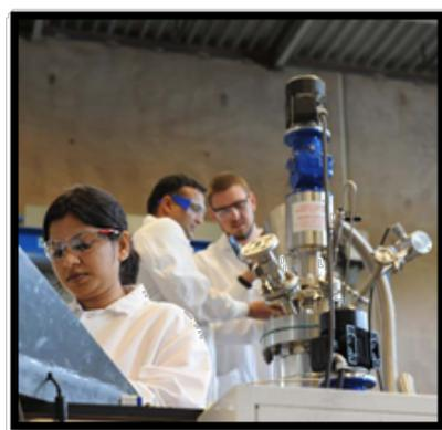
WSU Bench—Scale pretreatment reactor (10L Reactor, 100L flash tank)
