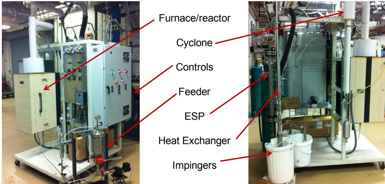
**Figure 1. RTI International's Bench-scale Hydrolysis Reactor System**
