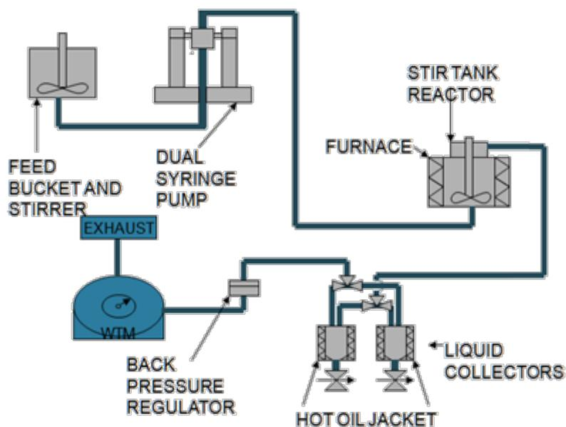
Figure 2. HTL reactor set-up at PNNL
