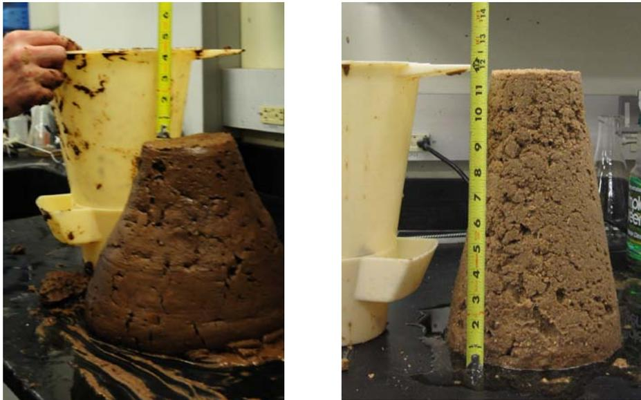
Figure 2. Slump-testing, immersion milled pine (left), 4 inch slump, and hammer milled corn stover (right), zero slump
