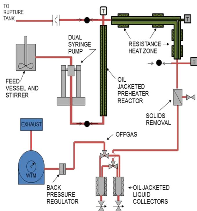
Figure 3. Process flow schematic of plug flow reactor system
