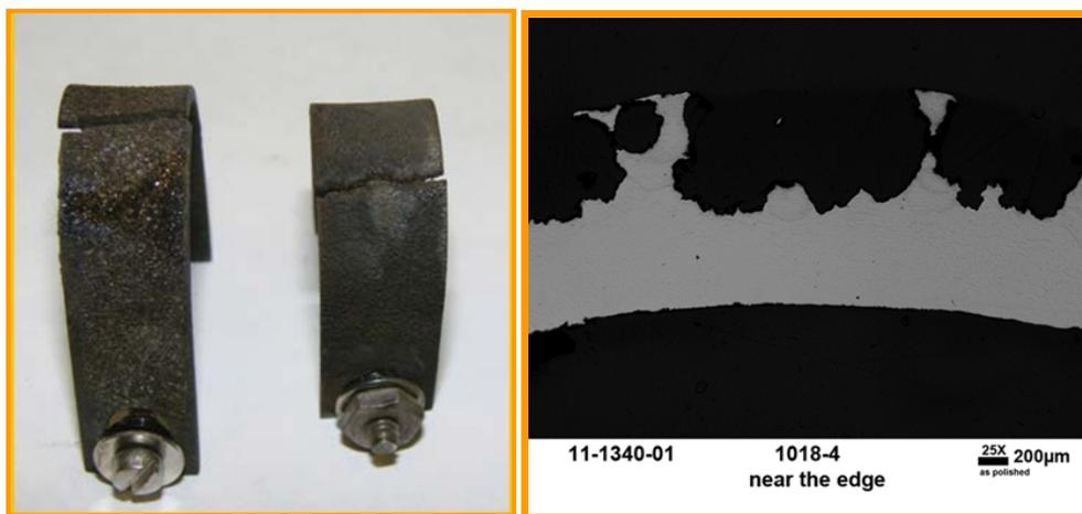
**Figure 3. Examples of stress corrosion cracked U-bend samples and cross section of a sample that experienced stress accelerated corrosion**
