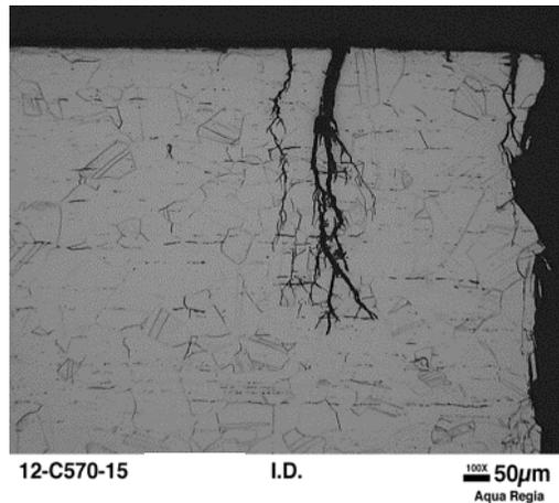
**Figure 4. Stress corrosion cracking seen in stainless steel fitting**
