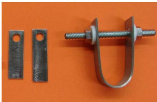
**Figure 2. General and U-bend stress corrosion cracking samples**
