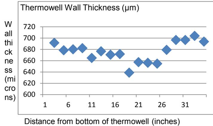
**Figure 6. Variation in wall thickness showing thinning near center of the thermowell**
