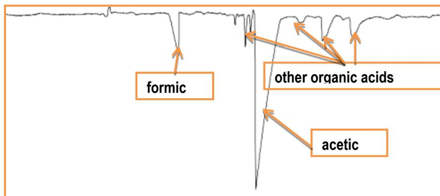
Figure 1. Example of capillary electrophoresis results identifying acid contents
