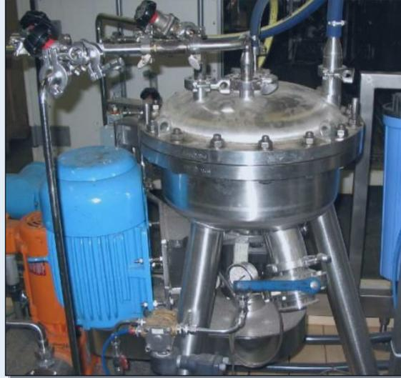
Pall Corporation constructed, shipped, and installed at NREL's facilities in Golden, Colorado, a crossflow filtration system based on the ZHF work and small scale laboratory crossflow testing. The system is designed to produce 2000 liters of sugar solution, filtered to less than 0.1  $\mu\text{m}$ , in 5-10 hours. This process can be scaled up to commercial scale. It is anticipated that the testing at NREL will lead to additional improvements to the design.
