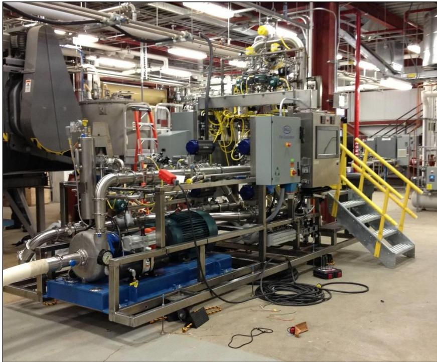
**Figure 3.** Hydrolysate is currently being produced for processing in this crossflow system. Small scale testing and Pall's knowledge of crossflow suggests that this process will be able to produce a high quality permeate in a cost effective manner.
