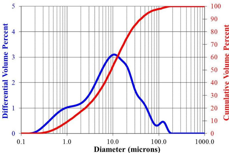
**Figure 1.** The large fraction of very small particles in the hydrolyzed biomass presents the greatest challenge to clarification because small particles produce a dense filter cake. A typical distribution is seen in this particle size distribution of hydrolyzed corn stover produced by the National Renewable Energy Laboratory (NREL) in 2012.
